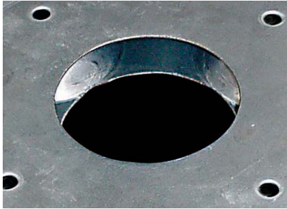
Step 1 Cut an 80mm diameter hole in the raised floor and carpet tile, lower the complete floor grommet into the cavity.
