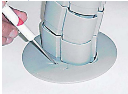
Step 5 To remove the Umbilical, place a screw driver in the slot provided. Press and hold down firmly and then remove umbilical.
